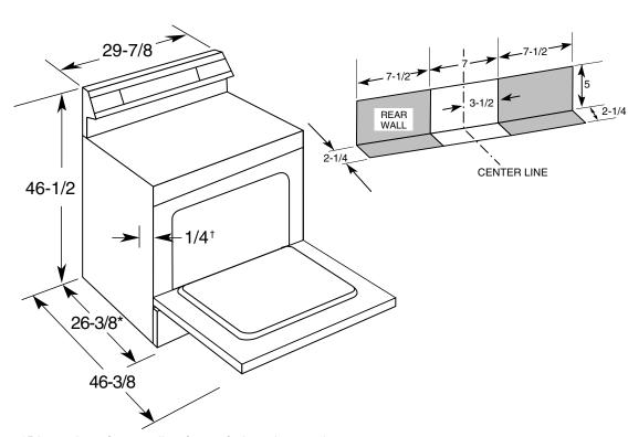
\*Dimensions from wall to front of closed oven door. Dimensions from wall to front of closed oven door handle is 28-1/2".
